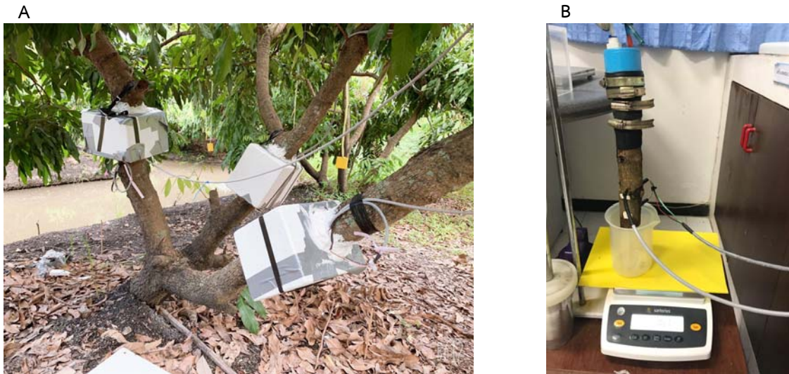
Figure 3 Sap flow installation: (A) field test with longan tree (B) calibration of single probe compared with commercial product.
